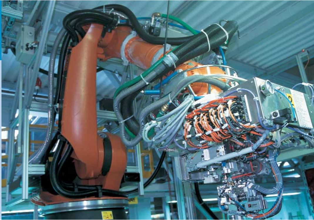
At the robot head, the Beckhoff I/O modules can fully utilize their advantages: compact, robust, light-weight.
