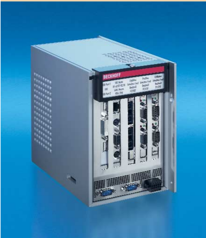
C6340: 5-slot Industrial PC for space-saving control cabinet mounting
