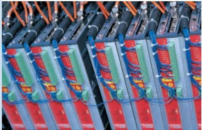
position and velocity. An incremental transducer signal having 1000 increments/24 mm is generated from their magnetic field strengths (24 mm corresponds to one logical rotation of the linear motor). Fed into the AX2000 drive amplifier, this yields a positioning accuracy of 0.1 mm.
