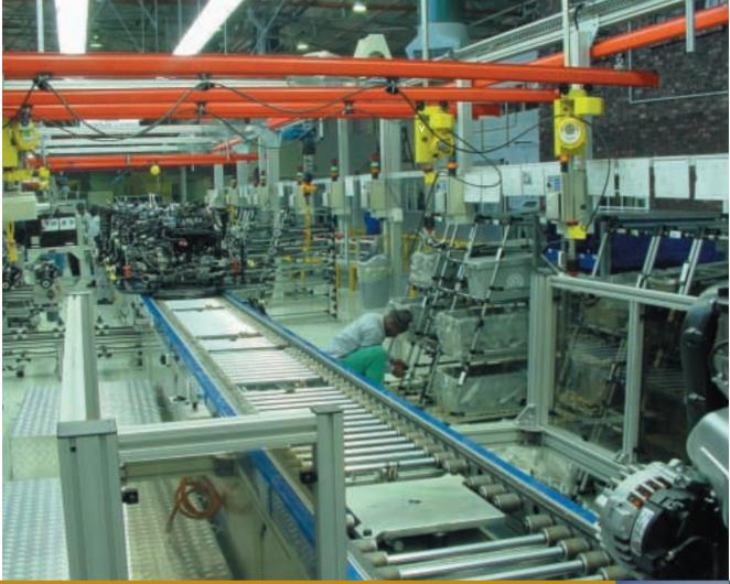
Over the last five years nearly all the assembly lines in the engine assembly area at the VW factory at Uitenhage in South Africa have been converted on the basis of PC-based control technology from Beckhoff. There are also TwinCAT controlled lines in final assembly and body shop. So far, more than 20 TwinCAT licenses and about 6000 I/O have been installed at Uitenhage. This ensures correct process reliability and data warehousing of all production processe
