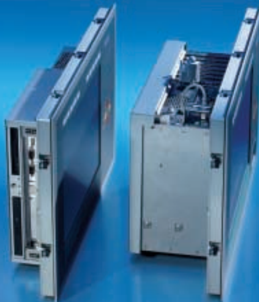
Panel PC = built-in Control Panel + add-on PC
