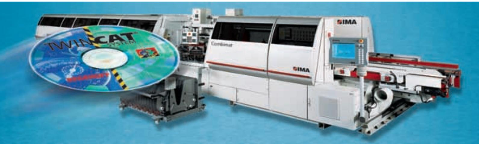
At the machine manufacturer IMA from Germany, the hardware PLCs have become redundant, since the company is now fitting PC-based controller equipment to all their woodworking machines. The first step has been taken with the Combimat edge processing machine.
