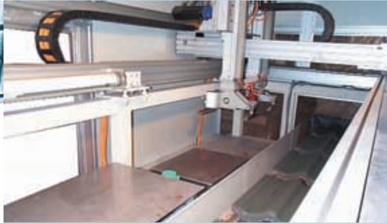
Inside view of the BSPK pilot plant, with test area, scales, gripper units and the production belt with roofing tiles.
