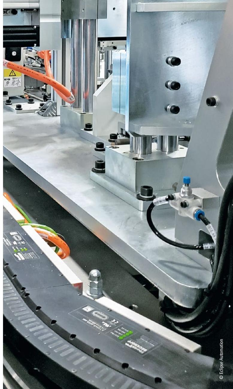
operators to quickly release and replace the pallet with a second type. This new pallet indexes forward and its specific position is measured to determine an offset. We apply those offsets to each individual pallet and make sure that components and parts line up exactly for the processes. So, the operator can easily load part type A, wait one cycle, and then load part type B with negligible downtime," Jeff Werner says.
