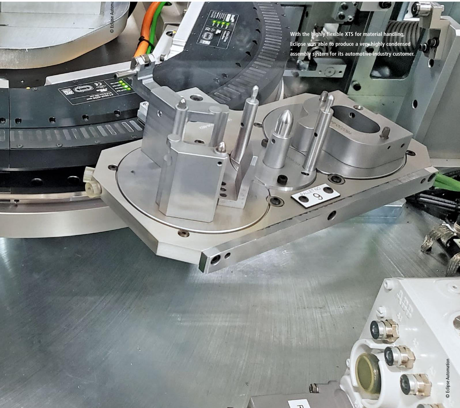
Three XTS systems ensure flexible material flow in the assembly line, ranging in sizes from 6 m track length with 12 movers to 12 m long with 18 movers.
