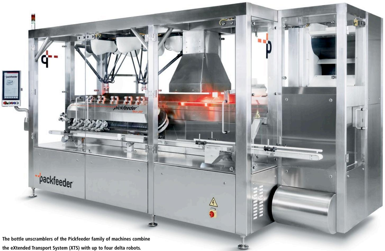
The bottle unscramblers of the Pickfeeder family of machines combine the eXtended Transport System (XTS) with up to four delta robots.
