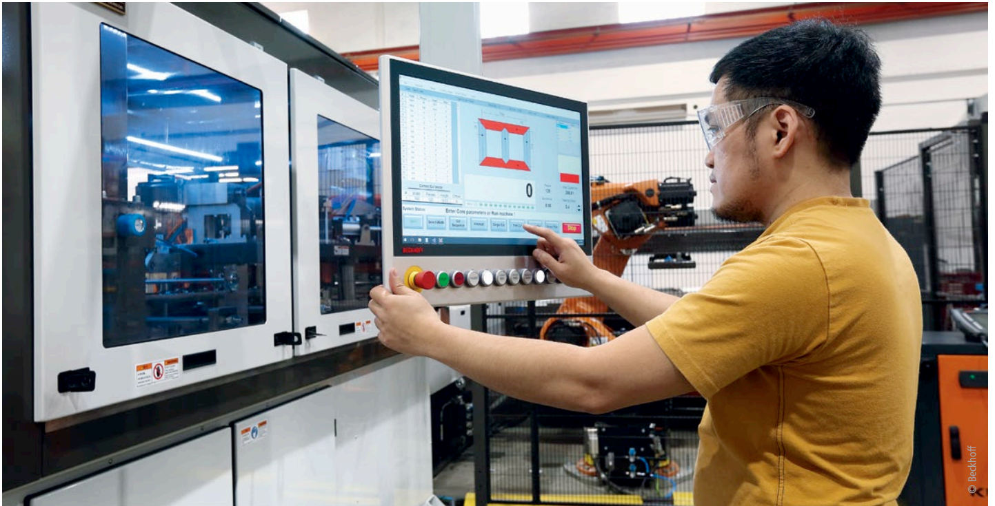
The 21.5-inch CP3921 multi-touch Control Panel with custom push-button extensions provides operator interface for the cutting cell, with a smaller touchscreen on the stacking cell.
