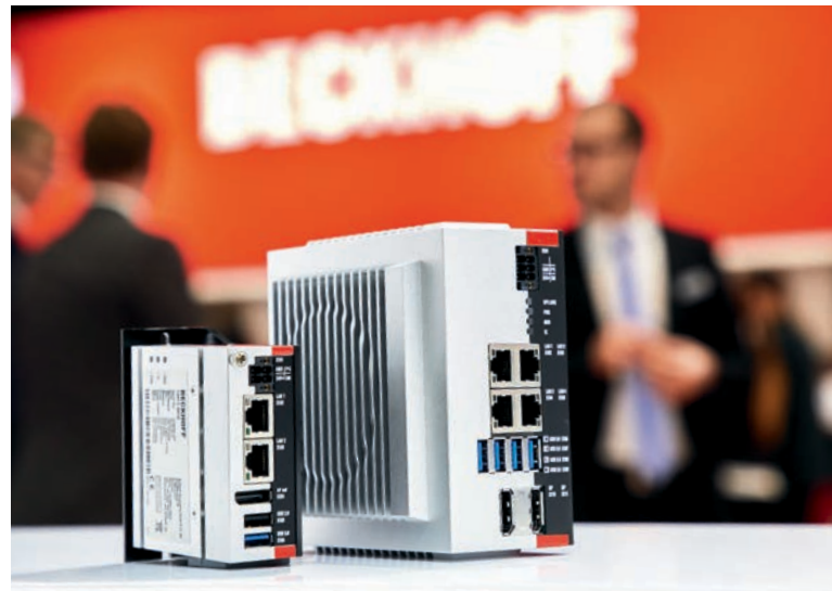
The C6030 Industrial PC (on the right) combines the ultra-compact design of the C6015 (on the left) with a very high level of computing power.
