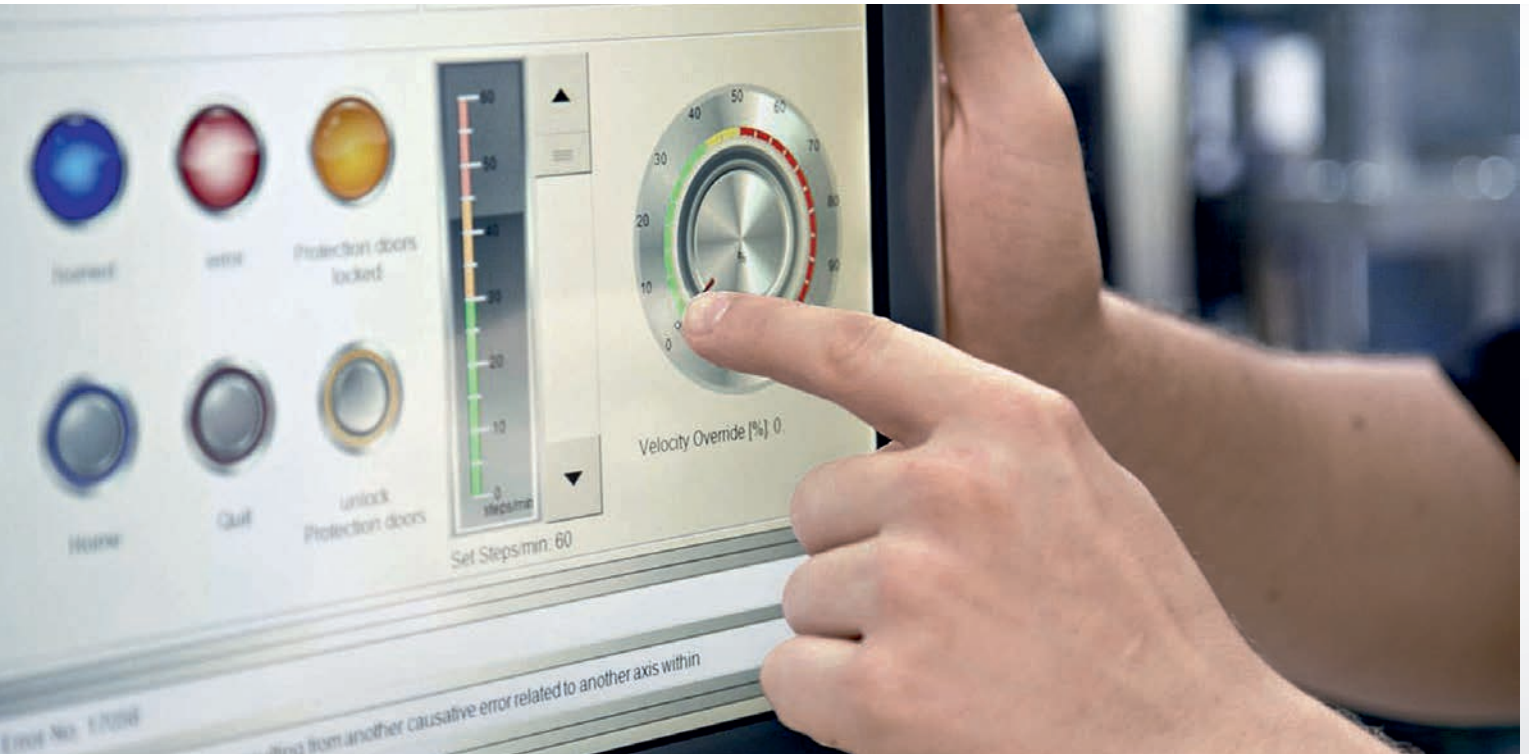
Leveraging the multi-touch functionality of the CP3919 Control Panel, a graphical rotary controller can be flexibly integrated via software.
