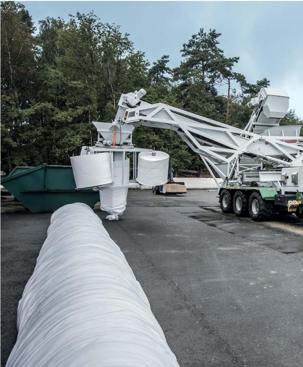
The picture shows the starting procedure when laying a second tube. Subsequently, a third hose is added in pyramid fashion. In this way, protective dams of a considerable size can be manufactured quickly using the Topomover 3.5.
