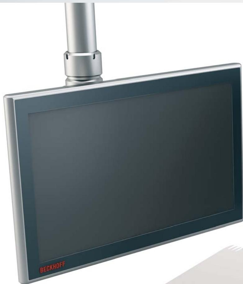
Designed for mounting arm installation, the CP32xx Panel PC series delivers multi-touch functionality and high computing power into the field in a single, advanced device.
