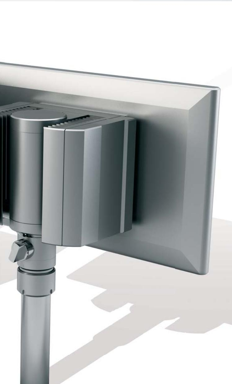
The area at the rear of the CP32xx Panel PC, which is required for swivelling and tilting the connected mounting arm, is also efficiently used to accommodate the added IPC components using little space. The components in this solution are thermally decoupled from each other: to save space, the computer is built around the integrated mounting arm in a u-shaped housing with cooling fins for passive cooling.
