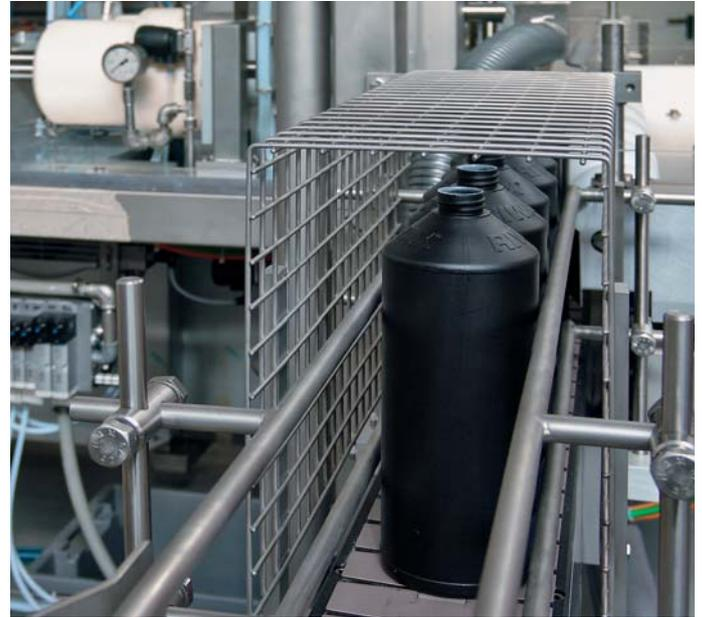
The polishing paste filling machine fills four 1kg containers simultaneously. The filling is done in a 12-second cycle.
