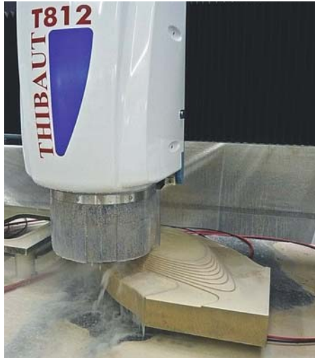
T812 CNC processing center for the manufacture of inner and outer contours, for the profiling and chamfer milling of curved or straight edges, for the surface grinding of marble and granite workpieces, and for drilling, thinning, sizing and groove milling.
