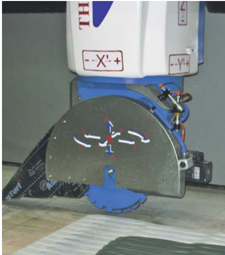
The T508 texture processing center from Thibaut handles polishing, matt grinding, antique brushing, gloss finishing and bush hammering of granite and other stone surfaces for interior decoration.
