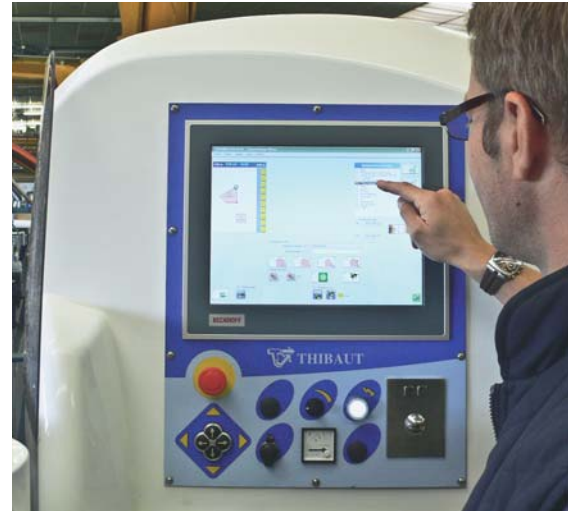
As a human-machine interface (HMI), the Beckhoff CP6202 'Economy' built-in Panel PC with 15-inch display permits more convenient operation of the processing center.
