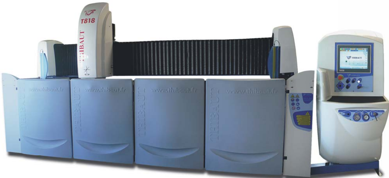
The T818 CNC processing center is available in different versions, for installation as a stand-alone machine or integrated into a production line. The machine optionally has a 3- or 4-axis controller and is designed for the manufacture of kitchen worktops with draining surfaces, washbasin covers, etc. from granite or marble. The machine includes a linear tool change magazine with two rows for 45 tools.
