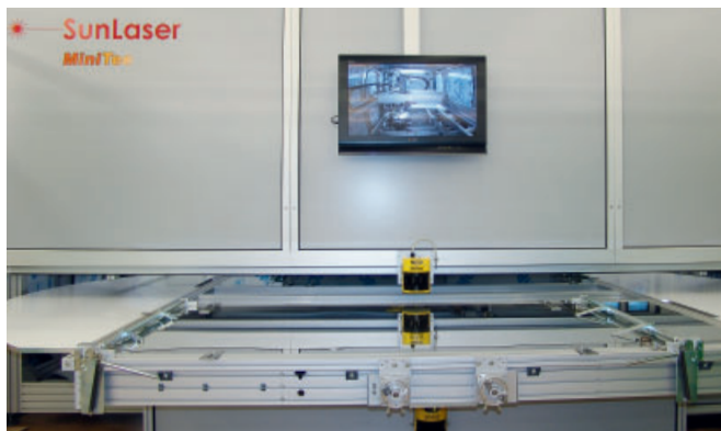
The SunLaser® flatbed laser welding system can be used to produce absorbers measuring 1,250 mm x 2,500 mm (4-ft x 8-ft).
