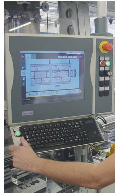
The Beckhoff Control Panel has a touch screen and is connected to the IPC via CP-Link.
