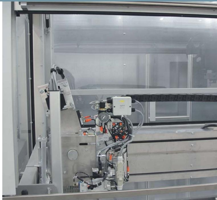
Dispensing unit in the contacting system: the highly precise application of the conductive adhesive is visually monitored. Dispensing is accomplished by a stepping motor controlled directly via a Beckhoff stepper motor terminal.
