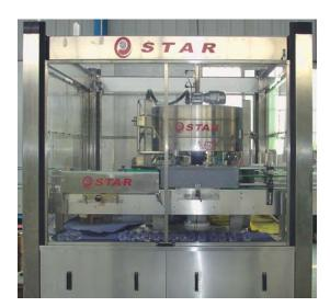
The E-Star hot-glue labeling machine can label between 24,000 and 48,000 bottles per hour.
