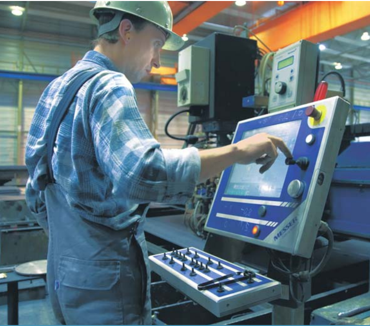
Machine operator at the operating panel of the flame cutting machine for the contour cut (l or vertical cut)
