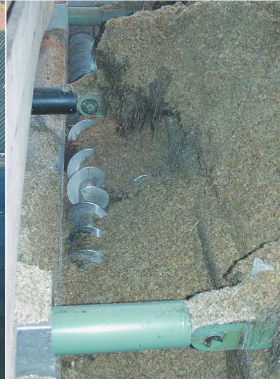
Feeding screws convey the biomass into the fermenters.
