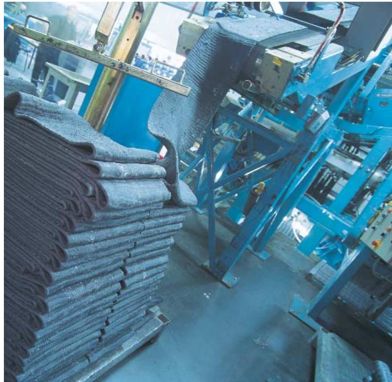
Semi-finished material is taken to one of three extruders
