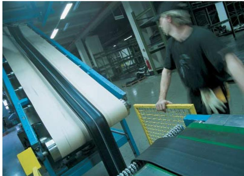
Treads after the cooling section, just before the cutting unit
