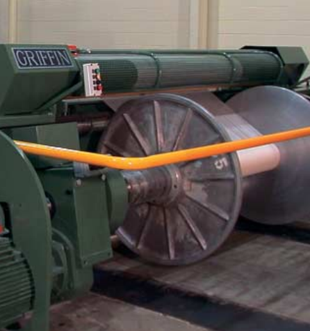
Top and right: Different views of sizing machines with Beckhoff control systems.
