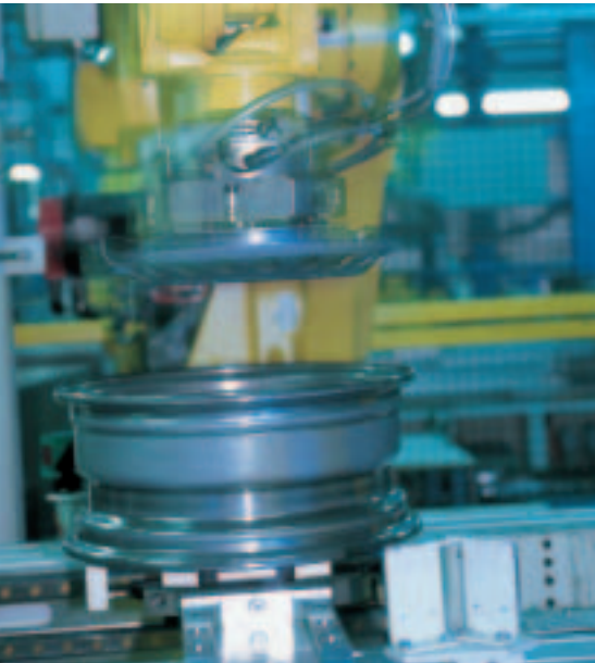
At the assembly machine, the wheel disc is inserted into the wheel rim.
