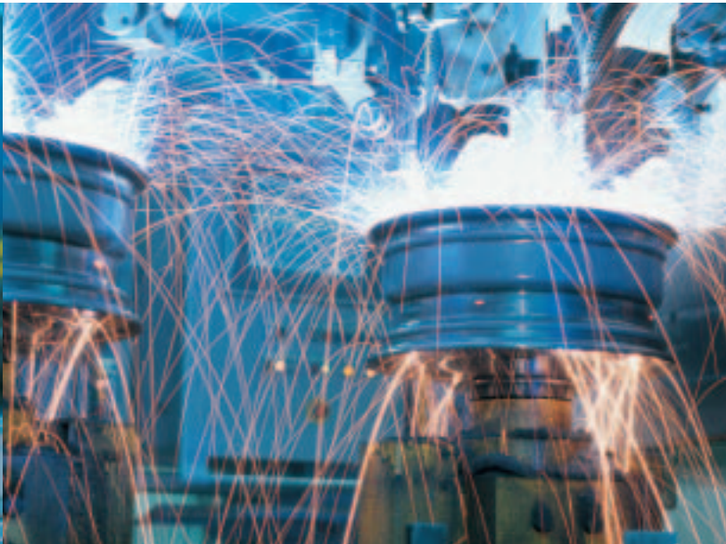
The final step: the welding of wheel disc and wheel rim.
