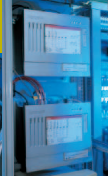
Beckhoff Industrial PC C6140 at the assembly machine with integrated Software PLC/NC TwinCAT.
