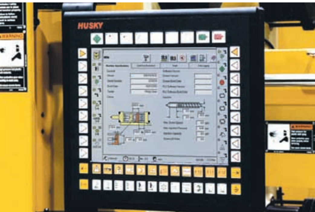
→ Control Panel with TFT display, touch screen, softkeys, and user ID system.
